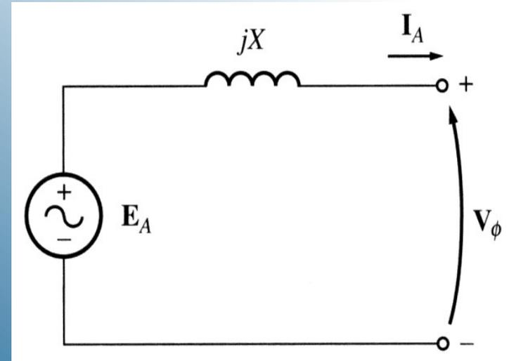
However, in addition to armature reactance effect, the stator coil has a self-inductance  $L_A$  ( $X_A$  is the corresponding reactance) and the stator has resistance  $R_A$ . The phase voltage is thus
