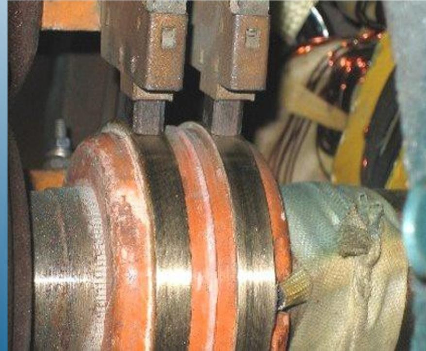
Slip rings are metal rings completely encircling the shaft of a machine but insulated from it. Graphite-like carbon brushes connected to DC terminals ride on each slip ring supplying DC voltage to field windings.
