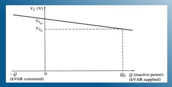
• Both the frequency-power and terminal voltage vs. reactive power characteristics are important for parallel operations of generators.
