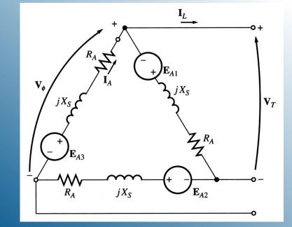
$V_T = V_{\phi} - for \Delta$
