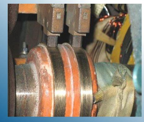
Slip rings are metal rings completely encircling the shaft of a machine but insulated from it. Graphite-like carbon brushes connected to DC terminals ride on each slip ring supplying DC voltage to field windings.
